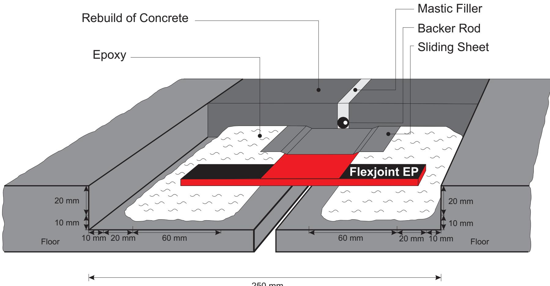
For a 2mm thick top and bottom bonding, approximately 2kg/m<sup>2</sup> of Epoxy is needed.
